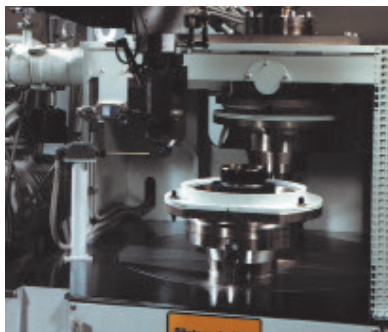
Electron-beam welding of diaphragm accumulators
