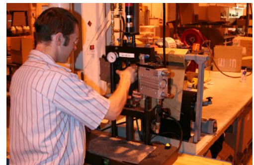
Precharging of a Diaphragm Accumulator
